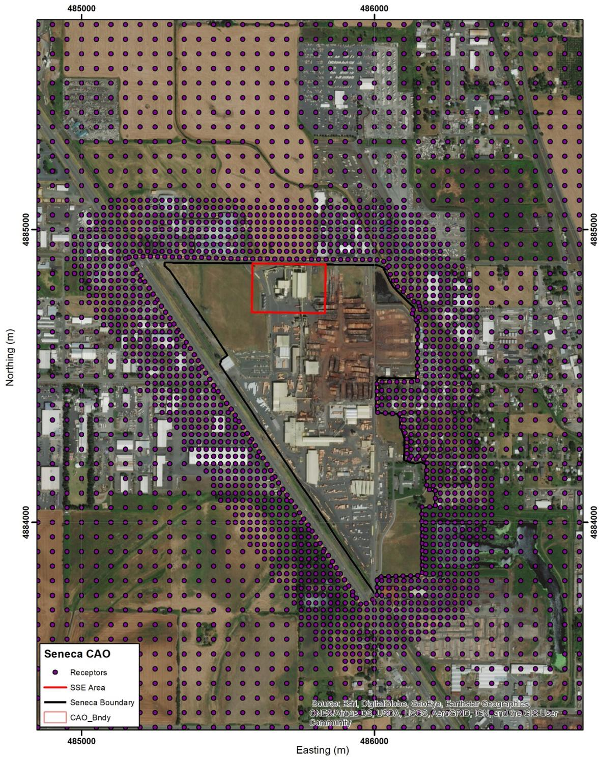
Figure 3-4: Far Field Receptor Grid
