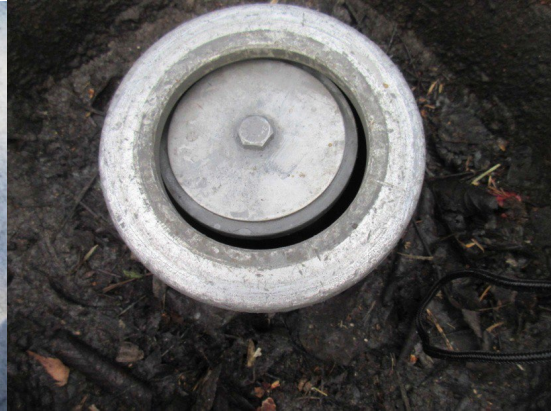
'Poppet Valve' not sealing
