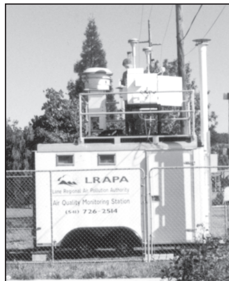
LRAPA monitoring site: one of three sites equipped to collect and log both pollution and meteorological data.
